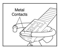
touching the lower contacts. Avoid moving your hands. After a moment, the heart-shaped indicator in the display will begin to flash and your heart rate will be shown. For the most accurate heart rate reading, continue to hold the contacts for about 15 seconds.
